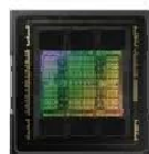
Hopper >80 billion transistors 814 mm 2 TSMC 4N
