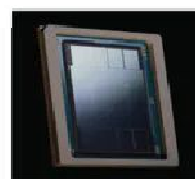
Blackwell >208 billion transistors >1600 mm 2 TSMC 4NP
